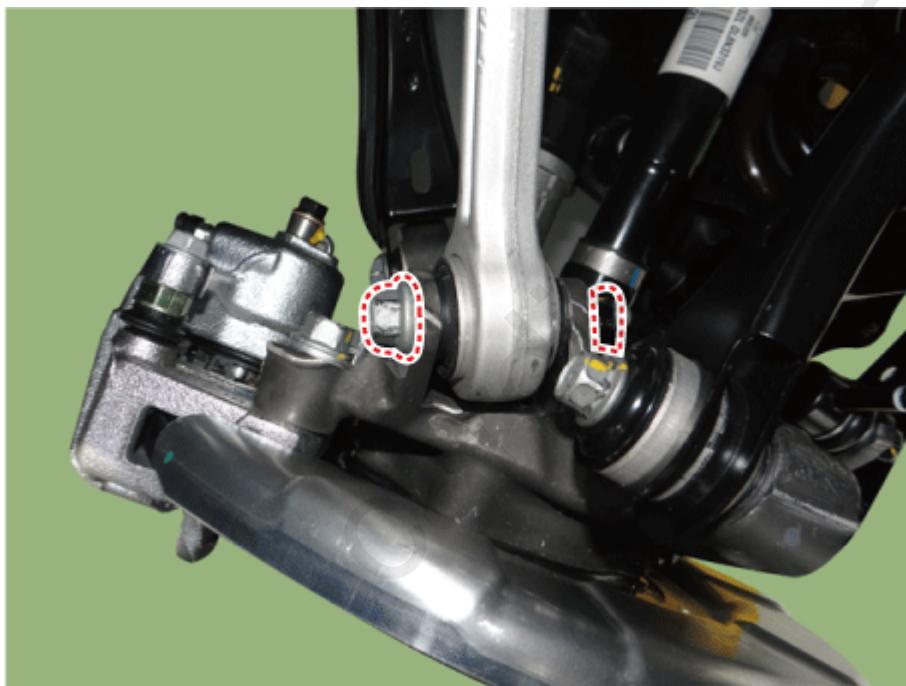
6. Loosen the rear shock absorber upper bolts and the remove the rear shock absorber.
